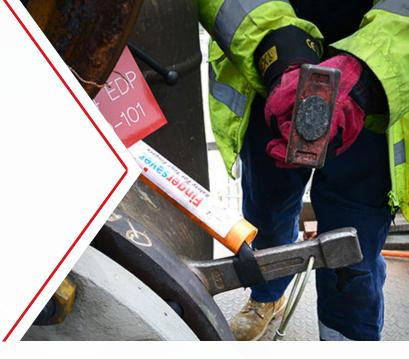
The MAXSafe Finger Saver Tool is intended to securely support and hold large spanners or flogging spanners in place during the removal of nuts and bolts.
