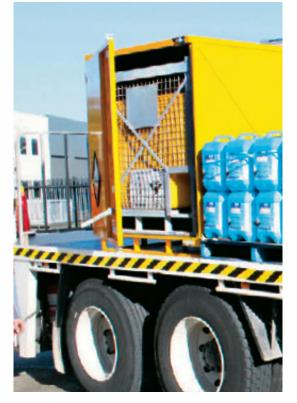
Example of SegBox used to facilitate legal transportation of incompatible chemical products on one truck. Note that you can also transport a 1000L IBC containing a packaging group II or III Dangerous Goods Rated Product using SegBox.
