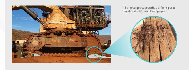
In this case, the client had been using timber slabs on their Excavator Lift Platforms which, when the machine is in place, tensions and raises the top of track to enable easier access to perform underbody maintenance.
